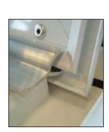
The sash must be held at about 95° to the plane of the roof to engage onto the hinge. Hook the outer channel, on the underside of the frame, onto the aluminium hinge as shown and rotate the sash to the closed position to engage the hinge.
